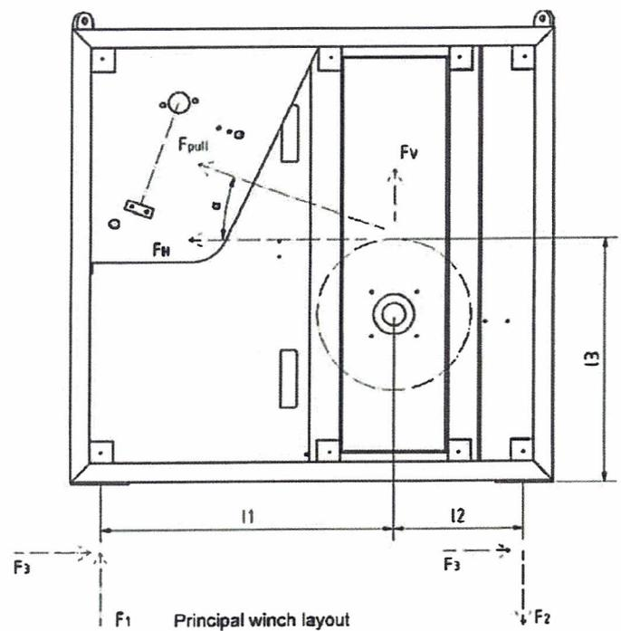
The following bolt holes reactions are calculated using MPT and valid for each individual bolt hole.
