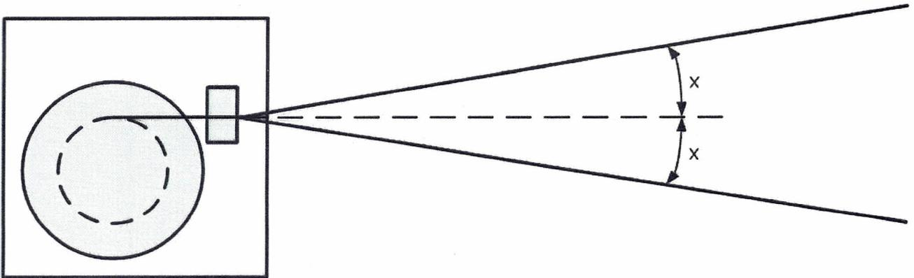
The horizontal fleet angle  $x$  is:  $\pm 8^\circ$
